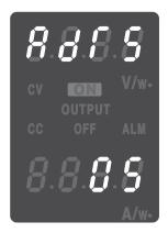
Fig.4-11Display example of node address "05"
