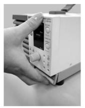
Fig.7-5 Removing the louver
