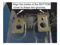
3. While holding the BOTTOM cover, insert the hook into the hole located above and to the left of the output terminal. At this point, pull the load cable from the hole on the near side of the terminal cover.
