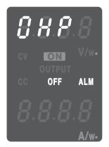
Fig.2-8 ALARM indication example (OHP)
